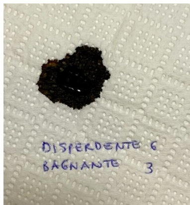
Figure 36 - Spot of carbon black dispersion with Diabolik dispersant at 6% and Diabolik humectant at 3%.
