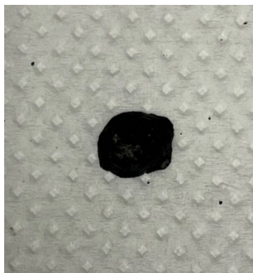
Figure 16 - Spot of carbon black dispersion with TEGO SML 20 MB.
