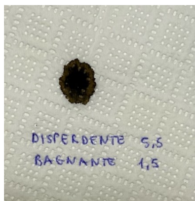
Figure 35 - Spot of carbon black dispersion with Diabolik dispersant at 5,5% and Diabolik humectant at 1,5%.
