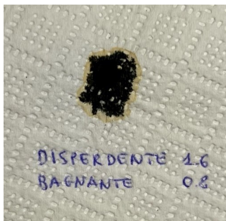
Figure 37 - Spot of carbon black dispersion with Diabolik dispersant at 1,6% and Diabolik humectant at 0,8%.
