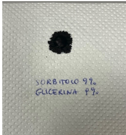
Figure 26 - Spot of carbon black dispersion with 9% of sorbitol and 9% of glycerin.
