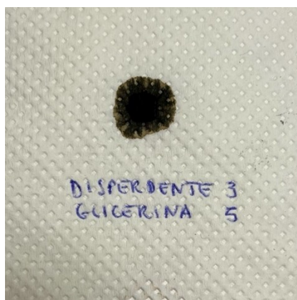
Figure 31 - Spot of carbon black dispersion with Diabolik dispersant at 3%.
