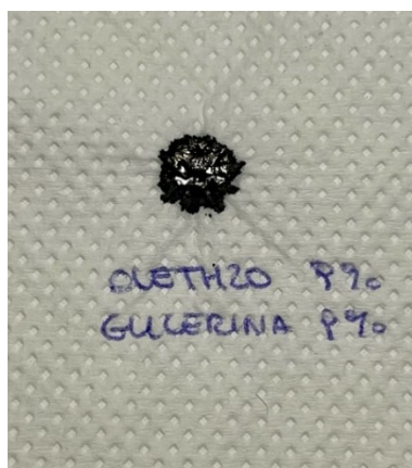
Figure 18 - Spot of carbon black dispersion with 9% of Oleth-20.
