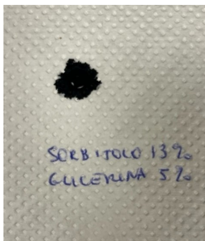
Figure 25 - Spot of carbon black dispersion with 13% of sorbitol and 5% of glycerin.
