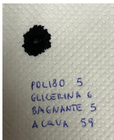
Figure 30 - Spot of carbon black dispersion with Diabolik humectant at 5% and TEGO SMO 80 at 5%.
