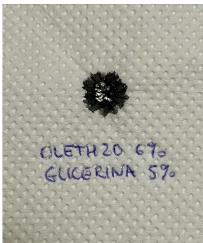
Figure 17 - Spot of carbon black dispersion with 6% of Oleth-20.
