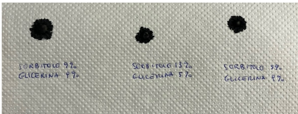
Figure 27 - Spots comparison among carbon black dispersions with different concentrations of sorbitol and glycerin.
