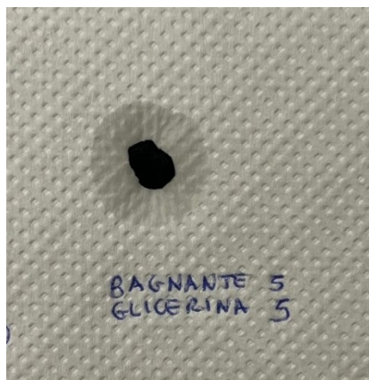
Figure 29 - Spot of carbon black dispersion with Diabolik humectant fixed at 5%.
