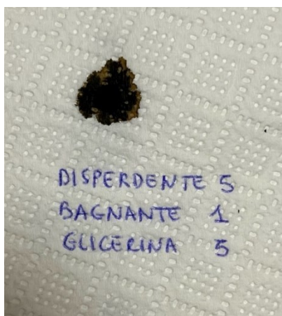
Figure 33 - Spot of carbon black dispersion with both Diabolik humectant and Diabolik dispersant fixed at 5%.
