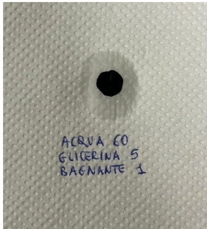
Figure 28 - Spot of carbon black dispersion with Diabolik humectant fixed at 10%.
