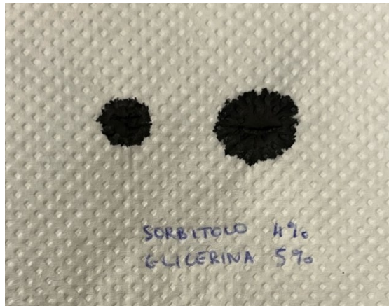
Figure 23 - Spot of carbon black dispersion with 4% of sorbitol and 5% of glycerin.
