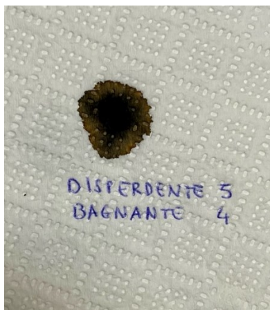
Figure 34 - Spot of carbon black dispersion with Diabolik dispersant at 5%, and Diabolik humectant at 4%.
