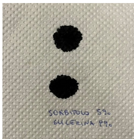
Figure 24 - Spot of carbon black dispersion with 5% of sorbitol and 9% of glycerin.
