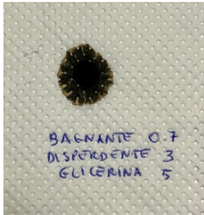
Figure 32 - Spot of carbon black dispersion with Diabolik dispersant at 3% and Diabolik humectant at 0.7%.
