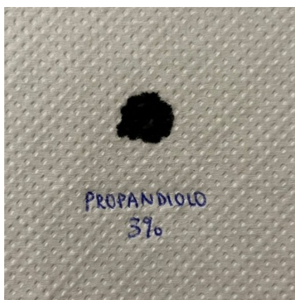
Figure 19 - Spot of carbon black dispersion with 3% of propanediol.
