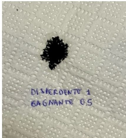
Figure 38 - Spot of carbon black dispersion with Diabolik dispersant at 1,0% and Diabolik humectant at 0,5%.
