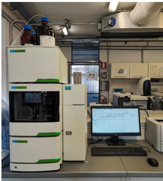
*Figura 13: strumento HPLC LC300 PerkinElmer.*
