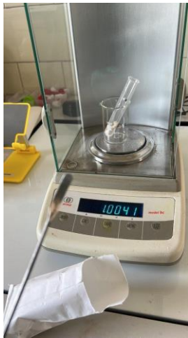
Figure 20: Weighing of wholemeal flour samples for DON extraction.
