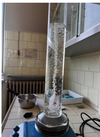
Figure 17: Preparation of 2% sodium dodecyl sulfate (SDS) solution used for SDS sedimentation analysis.
