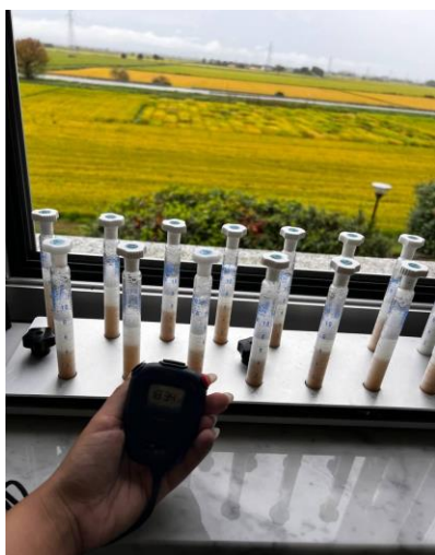
Figure 18: SDS Sedimentation Test showing final sediment volumes of wheat flour samples.
