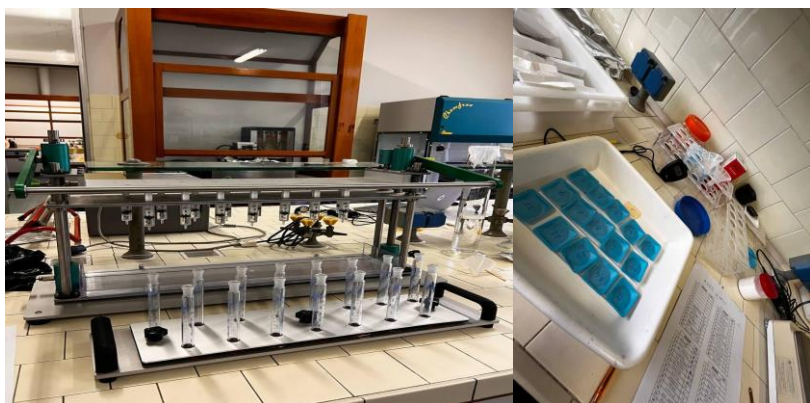
Figure 16: SDS-sedimentation apparatus for simultaneous analysis of 15 flour samples.
