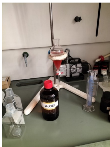
Figure 7. Purple cabbage liquid-liquid extraction
