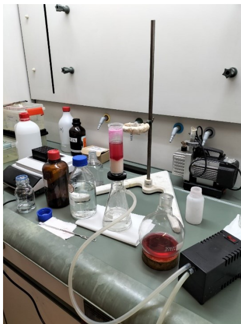
Figure 8. Purple cabbage purification on C18 Silica gel spherical
