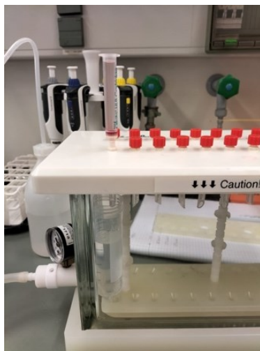
Figure 9. Purple cabbage purification on Oasis® HLB 3cc Vac cartridge
